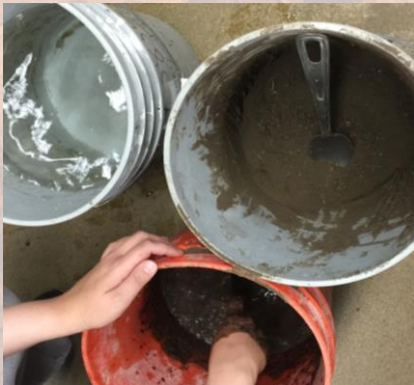
Fig 11: Mixing soil and water
