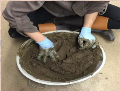
Fig 14: Mixing soil, water, and cement
